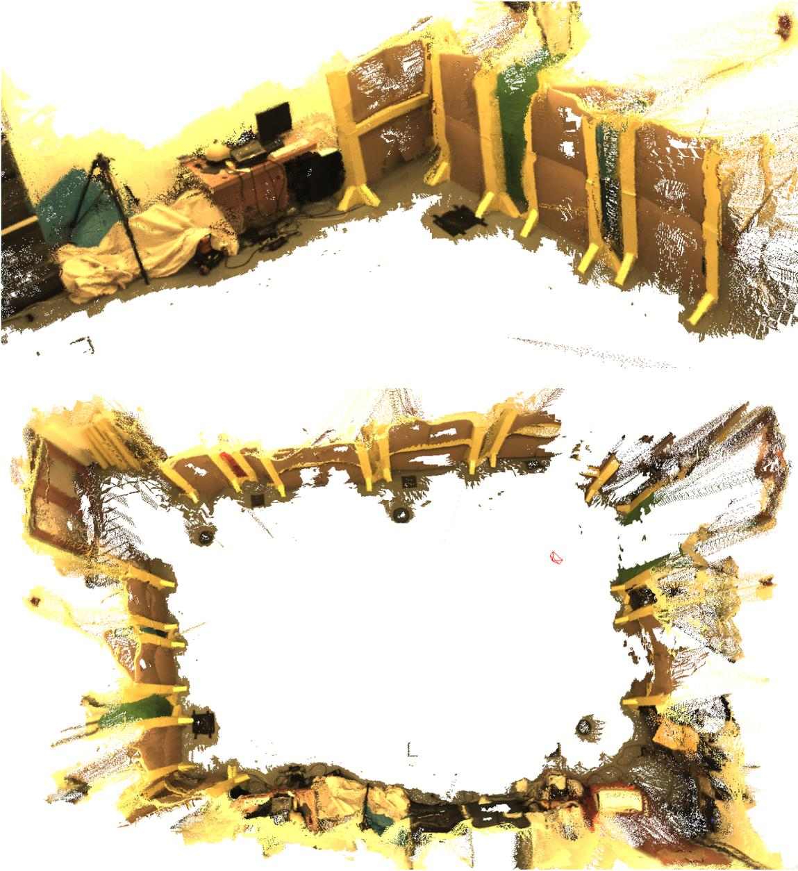
Figure 4-2: Our multi-level depth estimation and spatial regularization process enables dense point cloud maps to be generated online without GPU acceleration. This point cloud was generated in real-time from approximately two minutes of 30 Hz video around a laboratory workspace.
